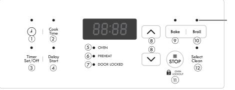
Function indicator lights - These lights located above the functions will glow when the function is active.
